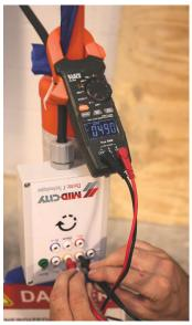
The Remote Voltage Verification Commissioning Box allows voltage reading of energized electrical equipment to happen without employees interacting directly with exposed energized electrical equipment.
